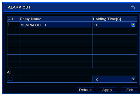
Fig 5-22 System Configuration-Alarm Out
