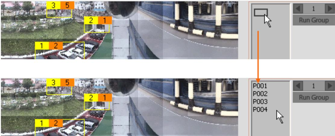
If you Click [Run Group], camera will move from a preset to other preset listed below repeatedly. If it arrive the last one, it will start from the beginning. It is noted that the interval will be determined by dwell time in the orange box and real moving time. To stop group operation, click [Run Group] button again.
