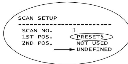
When scan function runs, camera moves from the preset assigned as the 1st point to the preset assigned as the 2nd point in CW(Clockwise) direction. Then camera moves from the preset assigned as the 2nd point to the preset assigned as the 1st point in CCW(Counterclockwise) direction. In case that the preset assigned as the 1st point is same as the preset assigned as the 2nd point, camera turns on its axis by 360° in CW direction and then it turns on its axis by 360° in CCW direction.
