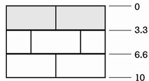
Camera has 6 BLC sensing zones on the screen. In BLC operation, The BLC sensing zone is used upper two zones on the screen like figure. At the BLC On setting, an object is distinguished more clearly in unfavorable light conditions by automatically controlling the video level.
