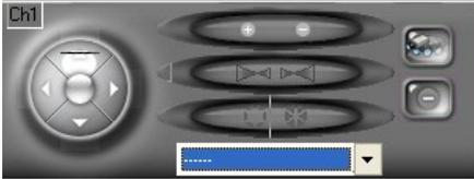
: PTZ controller interface. Provides Focus、Zoom、IRIS、Auto/ Stop Patrol and Preset Point control.
