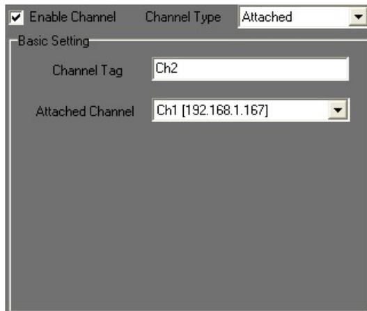
**Application of attached channel:** Attached channel type can operate with the digital zoom function. User can select different spots in the main channel and attach to different attached channels. Because attached channel type is not physically linked to any camera; such channel will not cost any loading of camera or HDD space. For instance, the following figure shows that CH2, 3 and 4 are only three parts of the CH1.
