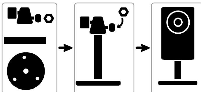
Step1: Fasten the base of the bracket (the round one) to where the camera is installed.
