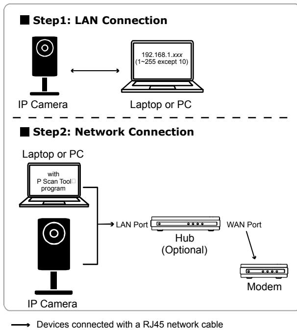
Step1: Disconnect your laptop / PC from the hub or modem, and connect it to this camera with a network cable.
