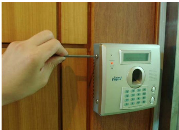
<Figure 3.5.15> how to attach the product to the plate
